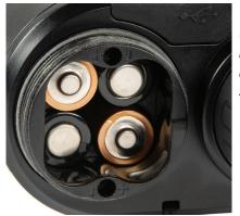
Batteries Installed (observe polarity marks inside compartment when installing batteries as shown here)
